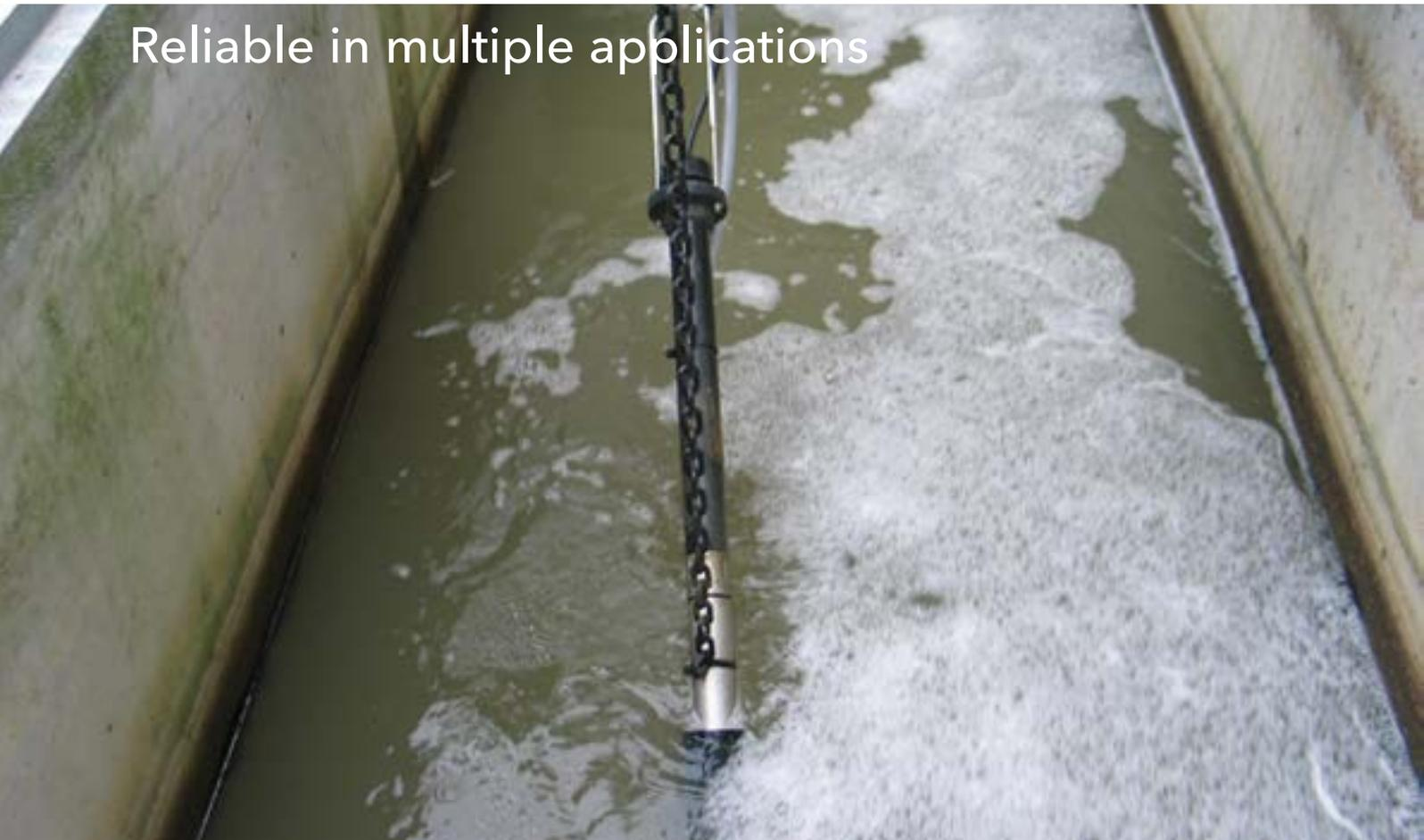
Conductivity is a well recognized and often indispensable parameter of state-of-the-art water, wastewater and industrial process analysis. Continuous measuring systems are employed to monitor the salt load of the influent in wastewater treatment plants, to control quality of drinking water and ultra-pure water or to determine non-specific contaminants in industrial processes.
