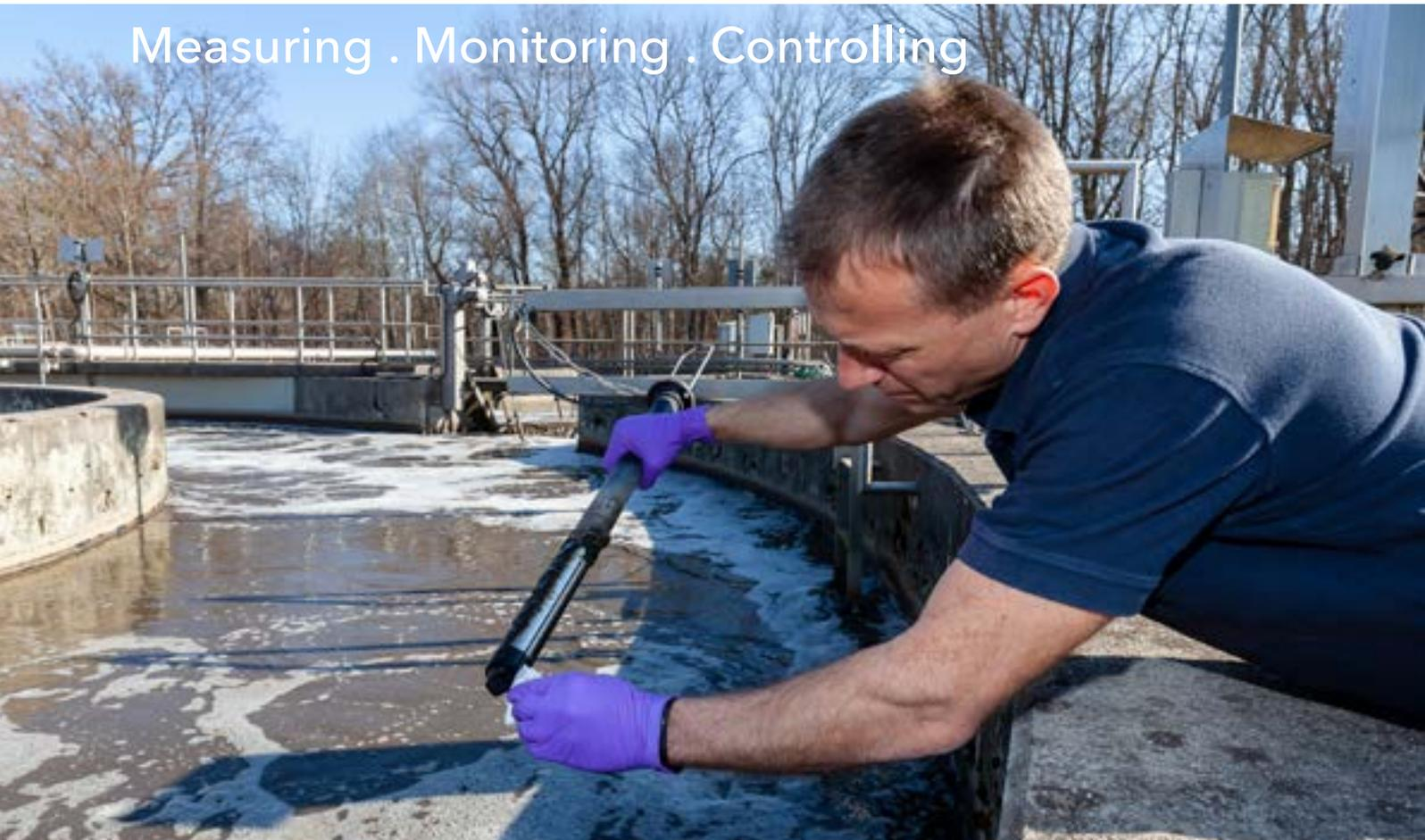
Reliable and continuous measurements of dissolved oxygen have become vitally important in many areas of the water/ wastewater treatment facilities. The availability of accurate and real-time measured concentrations is an absolute requirement for process monitoring and dynamic process control to ensure an efficient plant operation.
